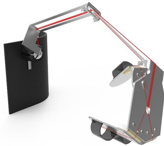
Fig. 4: Example of a locked position of the support arm
